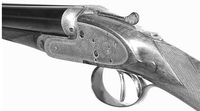
The action bottom (no floorplate!) shows the traditional rose-and-scroll engraving hand cut into all Purdeys, unless the buyer wanted something different. This gun still has most of its case colors.
