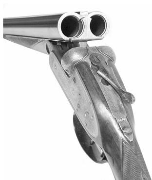
The self-opening action of the Purdey makes all other guns seem to have something missing. Pressing over the top lever causes the gun to open fully, remain fully open, and forcibly eject the empties. Closing it takes a distinct effort, a knack easily learned. The safety was automatic.
